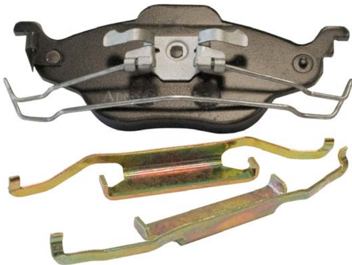
Replace springs and shims when fitting new pads to reduce NVH.
